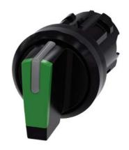
Selector switch, illuminable, 22 mm, round, plastic, green, selector switch, short, 3 switch positions I>O<II, momentary contact type, actuating angle  $2x45^{\circ}$ , 10:30h/12h/13:30h, with laser labeling, upper case
