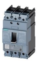
circuit breaker 3VA5 UL frame 125 breaking capacity class M 35kA @ 480 V 3-pole, line protection TM230, FTAM, In=125A overload protection Ir=125A fixed short-circuit protection Ii=5...10 x In cable connection on both sides
