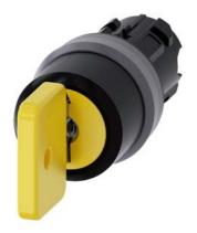
Key-operated switch O.M.R, 22 mm, round, plastic with metal front ring, lock number 73033, yellow, with 2 keys, 3 switch positions I-O-II, latching, actuating angle 2x45°, 10:30h/12h/13:30h, Key removal I+O+II, with laser labeling, inscription or symbol Customer-specific selection with SIRIUS ACT configurator (CIN)
