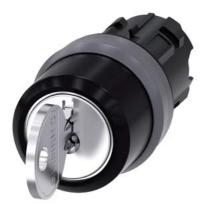
RONIS key-operated switch, 22 mm, round, plastic with metal front ring, lock number SB30, with 2 keys, 3 switch positions I-O-II, latching, actuating angle 2x45°, 10:30h/12h/13:30h, key removal O, possible special locks: SB31, 421, 455, with laser labeling, upper case and lower case, always upper case at the beginning of the word
