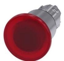
Illuminated mushroom pushbutton, 22 mm, round, metal, shiny, red, 40 mm, 3 switch positions, latches after pushing in, unlatches by pull-tounlatch mechanism to center position, after pulling out the button Retraction to center position, with laser labeling, upper case
