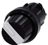
Selector switch, 22 mm, round, plastic, white, Rotary knob, 4 switch positions I-II-III-IV, latching, Actuating angle 4x90°, 3h/6h/9h/12h, with laser labeling, inscription or symbol Customer-specific selection with SIRIUS ACT configurator (CIN)
