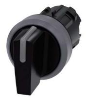
Illuminable selector switch, 22 mm, round, plastic with metal front ring, black, Selector switch short, 3 switch positions I-O-II, latching, actuating angle 2x45°, 10:30 /12 /13:30, Z=50-unit packaging
