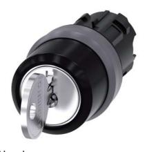
RONIS key-operated switch, 22 mm, round, plastic with metal front ring, lock number SB30, with 2 keys, 3 switch positions I-O<II, left latching, right momentary contact type, actuating angle 2x45°, 10:30h/12h/13:30h, key removal I, possible special locks: SB31, 421, 455, with laser labeling, upper case and lower case, always upper case at the beginning of the word
