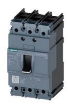
circuit breaker 3VA5 UL frame 125 breaking capacity class S 25kA @ 480 V 3-pole, line protection TM210, FTFM, In=125A overload protection Ir=125A fixed short-circuit protection Ii=10 x In UL489 SB (naval), 50 deg. cel. nut keeper kit on both sides
