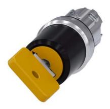
Key-operated switch O.M.R, 22 mm, round, metal, shiny, lock number 73033, yellow, with 2 keys, 2 switch positions O-I, latching, actuating angle 90°, 10:30h/13:30h, key removal O, with laser labeling, upper case and lower case, always upper case at beginning of line
