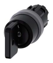
Key-operated switch O.M.R, 22 mm, round, plastic with metal front ring, lock number 73034, black, with 2 keys, 3 switch positions I-O<II, left latching, right momentary contact type, actuating angle 2x45°, 10:30h/12h/13:30h, key removal I, with laser labeling, upper case
