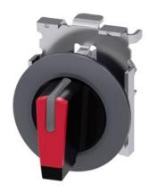
Selector switch, illuminable, 30 mm, round, Metal, matte, red, selector switch, short, front ring for flush installation, 3 switch positions I>O<II, momentary contact type, actuating angle 2x45°, 10:30h/12h/13:30h, with laser labeling, inscription or symbol Customer-specific selection with SIRIUS ACT configurator (CIN)
