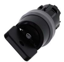
Key-operated switch O.M.R, 22 mm, round, plastic with metal front ring, lock number 73034, black, with 2 keys, 2 switch positions O<I, momentary contact type, Actuating angle 45°, 10:30h/12h, key removal O, Z=50-unit packaging
