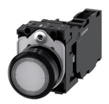
Illuminated pushbutton, 22 mm, round, plastic, clear, pushbutton, flat, momentary contact type, with holder, 1 NO+1 NC, LED module with integrated LED 110 V AC, screw terminal, with laser labeling, upper case and lower case, always upper case at beginning of line
