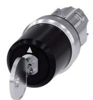
key-operated switch Siemens, 22 mm, round, metal, shiny, lock number SSG10, with 2 keys, 3 switch positions I>O<II, momentary contact on the left, latching on the right, actuating angle  $2x45^{\circ}$ , 10:30h/12h/13:30h, key removal II, with laser labeling, lower case
