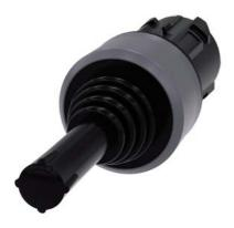
Coordinate switch, 22 mm, round, plastic with metal front ring, black, 4 switch positions, momentary contact type, without mechanical interlocking, Z=50-unit packaging
