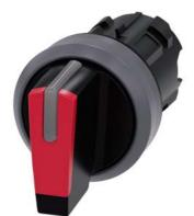
Selector switch, illuminable, 22 mm, round, plastic with metal front ring, red, selector switch, short, 3 switch positions I>O<II, momentary contact type, actuating angle 2x45°, 10:30h/12h/13:30h, with laser labeling, inscription or symbol Customer-specific selection with SIRIUS ACT configurator (CIN)
