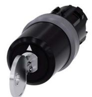
key-operated switch Siemens, 22 mm, round, plastic with metal front ring, lock number SSG10, with 2 keys, 3 switch positions I>O<II, momentary contact on the left, latching on the right, actuating angle 2x45°, 10:30h/12h/13:30h, key removal II Z=50-unit packaging
