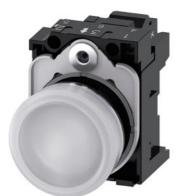
Indicator lights, 22 mm, round, metal, shiny, white, lens, smooth, with holder, LED module with integrated LED 24 V AC/DC, spring-type terminal, Z=20-unit packaging
