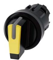
Selector switch, illuminable, 22 mm, round, plastic, yellow, selector switch, short, 3 switch positions I-O<II, left latching, right momentary contact type, actuating angle  $2x45^{\circ}$ , 10:30h/12h/13:30h, with laser labeling, upper case and lower case, always upper case at beginning of line
