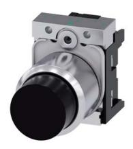
Pushbutton, compact, with extended stroke (12 mm), 22 mm, round, Metal, black, pushbutton, high, momentary contact type, with holder, with laser labeling, lower case
