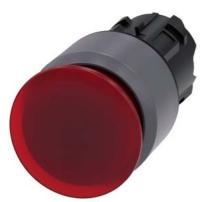
Illuminated mushroom pushbutton, 22 mm, round, plastic with metal front ring, red, 30 mm, latching, pull-to-unlatch mechanism, with laser labeling, upper case and lower case, always upper case at the beginning of the word
