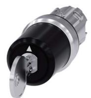
Key-operated switch BKS, 22 mm, round, metal, shiny, lock number S1, with 2 keys, 3 switch positions I-O<II, left latching, right momentary contact type, actuating angle  $2x45^{\circ}$ , 10:30h/12h/13:30h, key removal O, with laser labeling, upper case and lower case, always upper case at beginning of line
