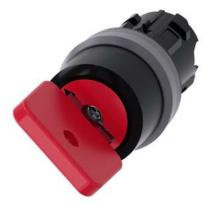
Key-operated switch O.M.R, 22 mm, round, plastic with metal front ring, lock number 73037, red, with 2 keys, 2 switch positions O-I, latching, actuating angle 90°, 10:30h/13:30h, key removal O+I, with laser labeling, upper case
