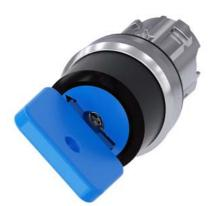
Key-operated switch O.M.R, 22 mm, round, metal, shiny, lock number 73038, blue, with 2 keys, 2 switch positions O-I, latching, actuating angle 90°, 10:30h/13:30h, key removal O+I, with laser labeling, inscription or symbol Customer-specific selection with SIRIUS ACT configurator (CIN)
