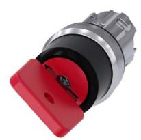
Key-operated switch O.M.R, 22 mm, round, metal, shiny, lock number 73037, red, with 2 keys, 2 switch positions O-I, latching, actuating angle 90°, 10:30h/13:30h, key removal O+I, with laser labeling, upper case
