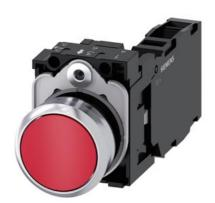
Pushbutton, 22 mm, round, metal, shiny, red, pushbutton, flat, momentary contact type, with holder, 1 NO+1 NC, screw terminal, with laser labeling, lower case
