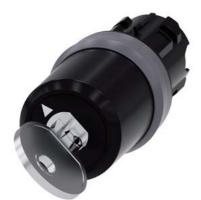
key-operated switch Siemens, 22 mm, round, plastic with metal front ring, lock number SSG10, with 2 keys, 2 switch positions O<I, momentary contact type, actuating angle 45°, 10:30h/12h, key removal O, with laser labeling, upper case
