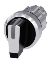
Selector switch, illuminable, 22 mm, round, metal, shiny, white, selector switch, short, 3 switch positions I>O<II, momentary contact type, actuating angle  $2x45^{\circ}$ , 10:30h/12h/13:30h, Z=50-unit packaging
