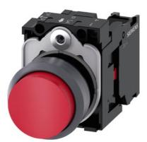
Pushbutton, 22 mm, round, plastic with metal front ring, red, pushbutton, raised, momentary contact type, with holder, 1 NC, screw terminal, with laser labeling, lower case
