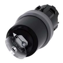
Key-operated switch IKON, 22 mm, round, plastic with metal front ring, lock number 360012K1, with 2 keys, 2 switch positions O-I, latching, actuating angle  $90^\circ, 10:30h/13:30h$ , key removal O, with laser labeling, upper case and lower case, always upper case at the beginning of the word
