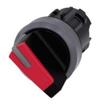
Selector switch, illuminable, 22 mm, round, plastic with metal front ring, red, selector switch, short, 2 switch positions O<I, momentary contact type, Actuating angle 45°, 10:30h/12h, with laser labeling, inscription or symbol Customer-specific selection with SIRIUS ACT configurator (CIN)
