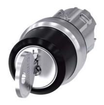
RONIS key-operated switch, 22 mm, round, metal, shiny, special lock, with 2 keys, 3 switch positions I-O-II, latching, actuating angle 2x45°, 10:30h/12h/13:30h, Key removal II, possible special locks: SB31, 421, 455
