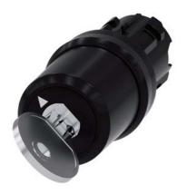
Key-operated switch BKS, 22 mm, round, plastic, Lock No. E7 (VW), without key, 2 switch positions O-I, latching, actuating angle 90°, 10:30h/13:30h, key removal O+I, with laser labeling, lower case
