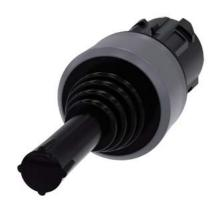
Coordinate switch, 22 mm, round, plastic with metal front ring, black, 4 switch positions, momentary contact type, without mechanical interlocking, with laser labeling, lower case
