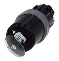
Key-operated switch BKS, 22 mm, round, plastic with metal front ring, lock number S1, with 2 keys, 2 switch positions O-I, latching, actuating angle 90°, 10:30h/13:30h, key removal I, with laser labeling, inscription or symbol Customer-specific selection with SIRIUS ACT configurator (CIN)
