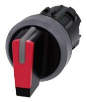
Selector switch, illuminable, 22 mm, round, plastic with metal front ring, red, selector switch, short, 3 switch positions I>O<II, momentary contact type, actuating angle  $2x45^{\circ}$ , 10:30h/12h/13:30h, with laser labeling, lower case
