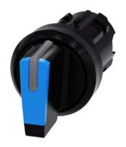
Selector switch, illuminable, 22 mm, round, plastic, blue, selector switch, short, 3 switch positions I>O<II, momentary contact type, actuating angle  $2x45^{\circ}$ , 10:30h/12h/13:30h, with laser labeling, upper case
