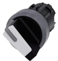
Selector switch, illuminable, 22 mm, round, plastic with metal front ring, white, selector switch, short, 2 switch positions O-I, latching, actuating angle 90°, 10:30h/13:30h, with laser labeling, lower case
