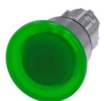
Illuminated mushroom pushbutton, 22 mm, round, metal, shiny, green, 40 mm, latching, pull-to-unlatch mechanism, with laser labeling, upper case and lower case, always upper case at beginning of line
