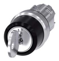
RONIS key-operated switch, 22 mm, round, metal, shiny, lock number SB30, with 2 keys, 3 switch positions I>O<II, momentary contact type, actuating angle 2x45°, 10:30h/12h/13:30h, key removal O, possible special locks: SB31, 421, 455, with laser labeling, upper case
