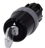
key-operated switch Siemens, 22 mm, round, plastic with metal front ring, lock number SSG10, with 2 keys, 3 switch positions I-O-II, latching, actuating angle 2x45°, 10:30h/12h/13:30h, key removal II, with laser labeling, lower case
