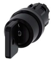
Key-operated switch O.M.R, 22 mm, round, plastic, lock number 73034, black, with 2 keys, 3 switch positions I-O<II, left latching, right momentary contact type, actuating angle 2x45°, 10:30h/12h/13:30h, Key removal I Z=50-unit packaging
