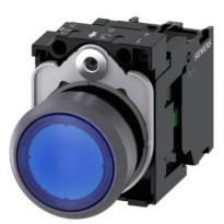
Illuminated pushbutton, 22 mm, round, plastic with metal front ring, blue, pushbutton, flat, momentary contact type, with holder, 1NO, LED module with integrated LED 24 V AC/DC, screw terminal, Z=20-unit packaging
