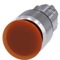
Illuminated mushroom pushbutton, 22 mm, round, metal, shiny, amber, 30 mm, latching, pull-to-unlatch mechanism, with laser labeling, upper case and lower case, always upper case at the beginning of the word
