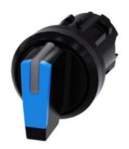
Selector switch, illuminable, 22 mm, round, plastic, blue, selector switch, short, 3 switch positions I>O<II, momentary contact on the left, latching on the right, actuating angle 2x45°, 10:30h/12h/13:30h, with laser labeling, inscription or symbol Customer-specific selection with SIRIUS ACT configurator (CIN)
