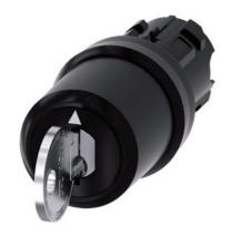
Key-operated switch IKON, 22 mm, round, plastic, lock number 360012K1, with 2 keys, 3 switch positions I-O-II, latching, actuating angle 2x45°, 10:30h/12h/13:30h, Key removal I+O+II, with laser labeling, lower case
