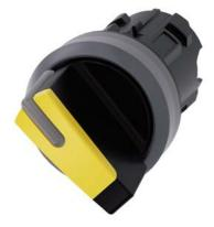
Selector switch, illuminable, 22 mm, round, plastic with metal front ring, yellow, selector switch, short, 2 switch positions O-I, latching, actuating angle 90°, 10:30h/13:30h, with laser labeling, upper case and lower case, always upper case at beginning of line
