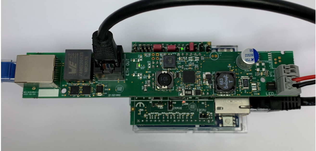
Figure 7. Operational NCL31010GEVK on Arduino UNO R3 and Arduino Ethernet Shield 2
