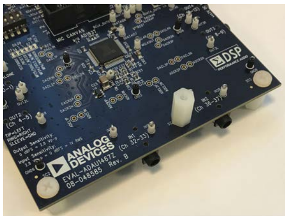
Figure 3. Nylon Screw and Standoff Fitted in Place
